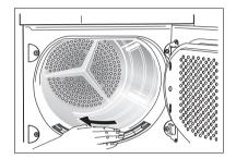
**3.** Push down unlock button on large mesh filter.
